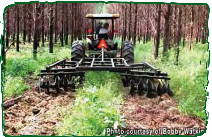
A slotted disk harrow which can straddle stumps can be used to disk the lanes until stump and wood debris has rotted enough for a regular disk to be used. (Consult with a local forestry professional prior to disking in areas where Annosum root disease is troublesome.)
